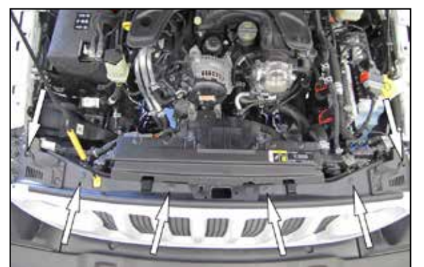
6. Remove the 6 clips at the top of the grill that secure grill to core support.
