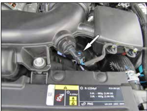
2. Disconnect the inlet air temp electrical connector.
