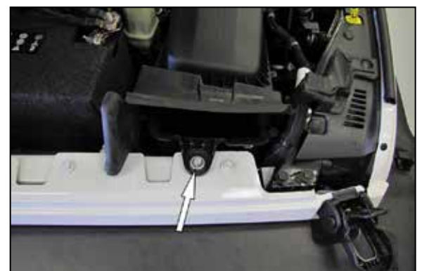
5. Remove the bolt that secures the factory air box to the fender and remove assembly from the vehicle.
