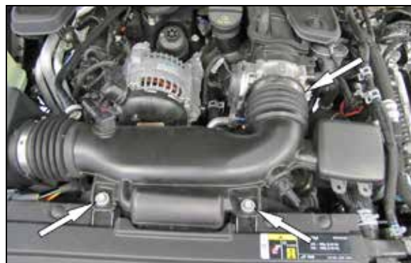
4. Remove the bolts that secure the factory tube to the fan shroud, then loosen hose clamp at throttle body.
