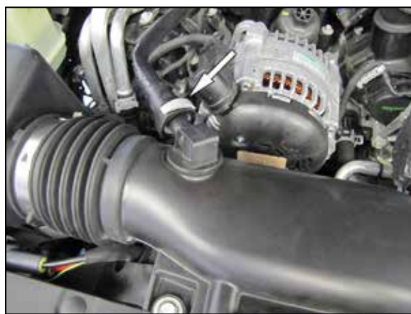
3. Disconnect the crank case vent line.
