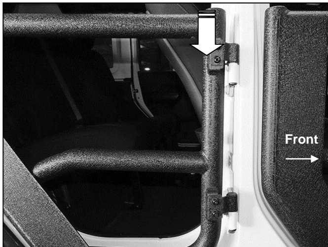
(Fig 10) Lift door, guide Hinge Pins down through hinge on vehicle. Slide end of Door Stop Strap onto bracket
